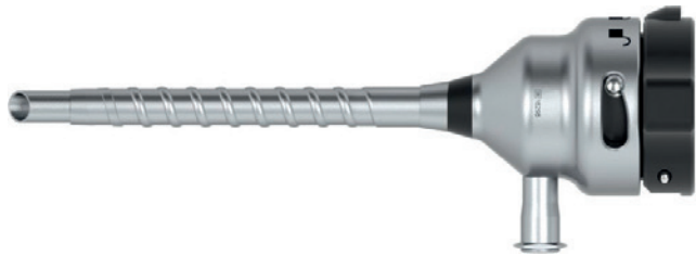
ELT-071F TROCAR SLEEVE with automatic silicone valve with fixation thread, with CO2 luer- lock connector*, Working length 60mm
